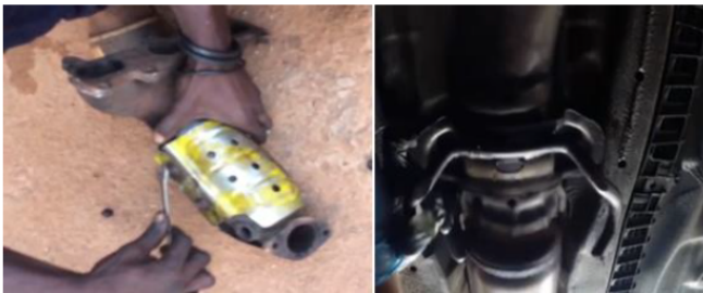
Figure 6: A refurbished catalytic converter adapted from [27]
